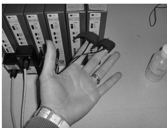
Figure 2 Location of the two skin conductance electrodes.
