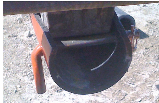
Figure 7: Fork pad securing
