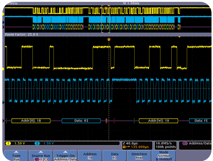
▶ Triggering on a specific data packet going across an I 2 C bus. Yellow waveform is data, blue waveform is clock. Bus waveform provides decoded packet content including Start, Address, Read/Write, Data, Missing Ack and Stop.
