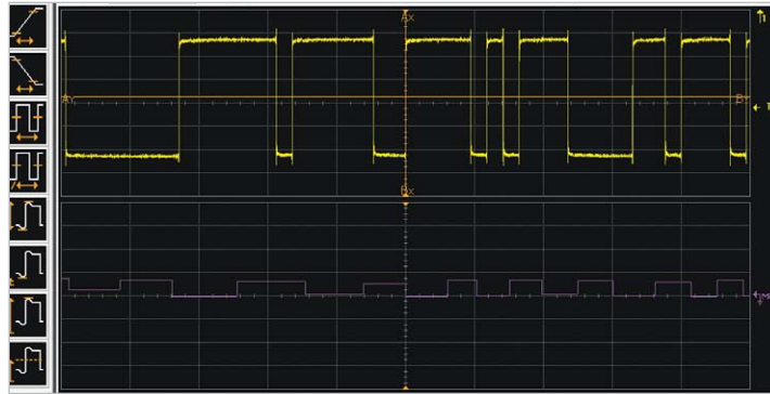
Figure 14. A trend display, showing a time plot of the measurement time-correlated with the signal waveform data, makes it easy to understand relationships between jitter and signal conditions.
