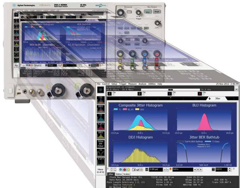
Figure 1. EZJIT Plus provides multiple views of jitter for maximum insight as well as quick, accurate separation of jitter subcomponents for compliance testing.
