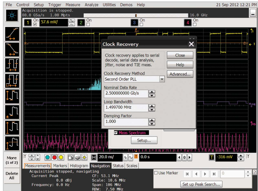
Figure 17. You can choose constant-frequency or phase-locked loop (PLL) clock recovery. With PLL clock recovery, the data rate, loop bandwidth and damping factor are adjustable.
