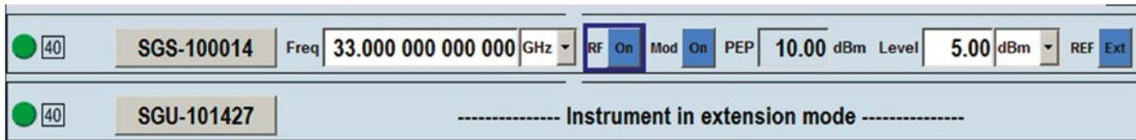
EVM performance measurement using the R&S®SGS100A/R&S®SGU100A combination driven by an R&S®AFQ100A at 14 GHz
