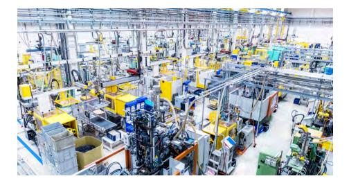
In a smart factory, cameras and sensors will be used to monitor and adjust manufacturing in real time. Costs can be reduced via lower error rates and less rework. Efficiency can be increased with improved throughput and less human intervention, leading to increased consistency and higher quality. (Source: Developers Alliance, Internet of Things, Manufacturing IoT From the Factory Floor.)
