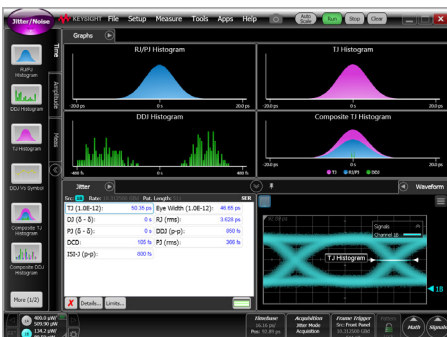
Jitter mode gives you insights into the root causes of both jitter and interference
