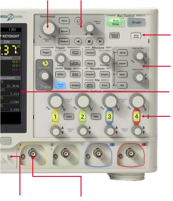
Autoscale lets you quickly display any analog or digital active signals, automatically setting the vertical, horizontal and trigger controls for the best display, while optimizing memory
