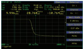
The markers show that te break point occurs approximately 20dB below the top of the pulse, equating to about 1% of the pulse power. With this in mind it should be noted that a pulse fall time is normally measured between the 90% and 10% levels, and so will not be influenced by this characteristic.
