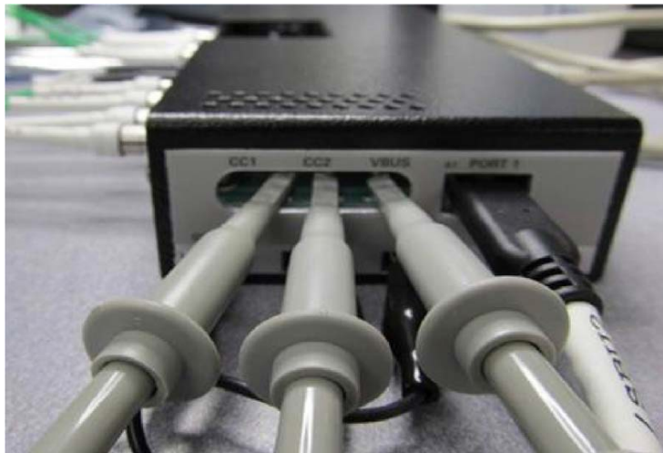
Figure 8. The CC1 and CC2 can be conveniently probed using a Keysight passive probe
