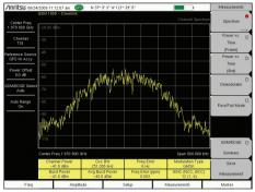
RF Measurement – Occupied Bandwidth
