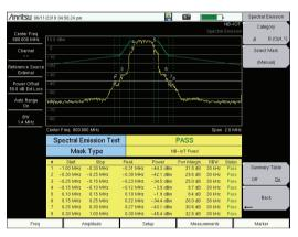
NB-IoT Analyzer Spectral Emission Mask
