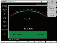
High Accuracy Power Meter (Option 0019) Requires external power sensor with convenient connection via a USB A/mini-B cable. Use upper/lower limit activation during pass/fail measurements.
