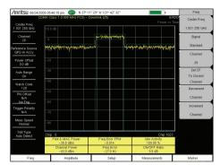
RF Measurements — Pilot and MAC Power High values will create pilot pollution. High or low values will cause dead spots/dropped calls and cell loading imbalances/blocked calls.
