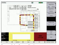
**On-screen Indoor Coverage Mapping** Import an image of an office floor plan and use the start-
