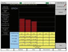
Over-the-Air Measurements – Scrambling Codes Too many strong sectors at the same location creates pilot pollution. This leads to low data rate, low capacity, and excessive soft handoffs.
