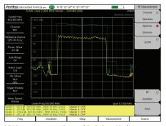
RF Measurements — Spectral Emissions Mask The 3GPP2 spectral emission mask is displayed. Failing this test leads to interference with neighboring carriers, legal liability, and low signal quality.
