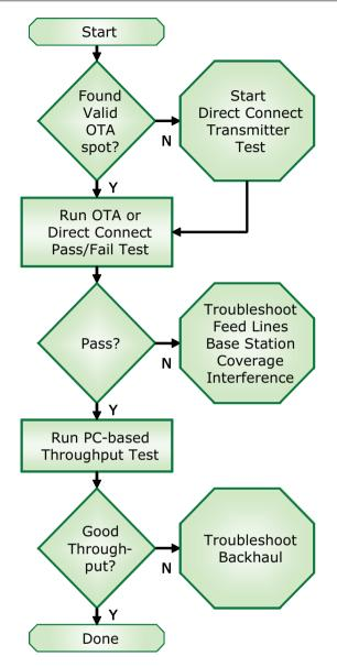
Fast Over-the-Air Pass/Fail Testing Process
