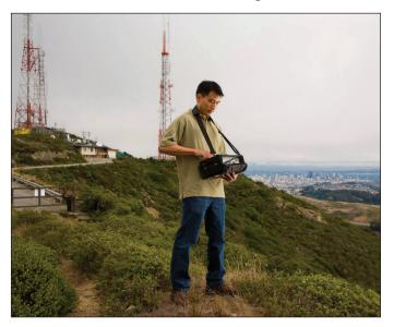
The BTS Master MT8220T feature an over-the-air (OTA) pass/fail test wireless measurement. Technicians and RF engineers can quickly determine the health of a cell site with a one-step pass/fail test that verifies the quality of:
