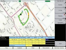
**OTA On-screen Mapping** Import map area on instrument screen to drive test downlink coverage of S-SS Power, RSRP, RSRQ, or SINR.
