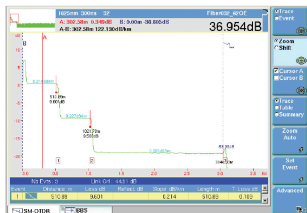
Figure 9: Sample OTDR output (Source: Viavi Solutions)
