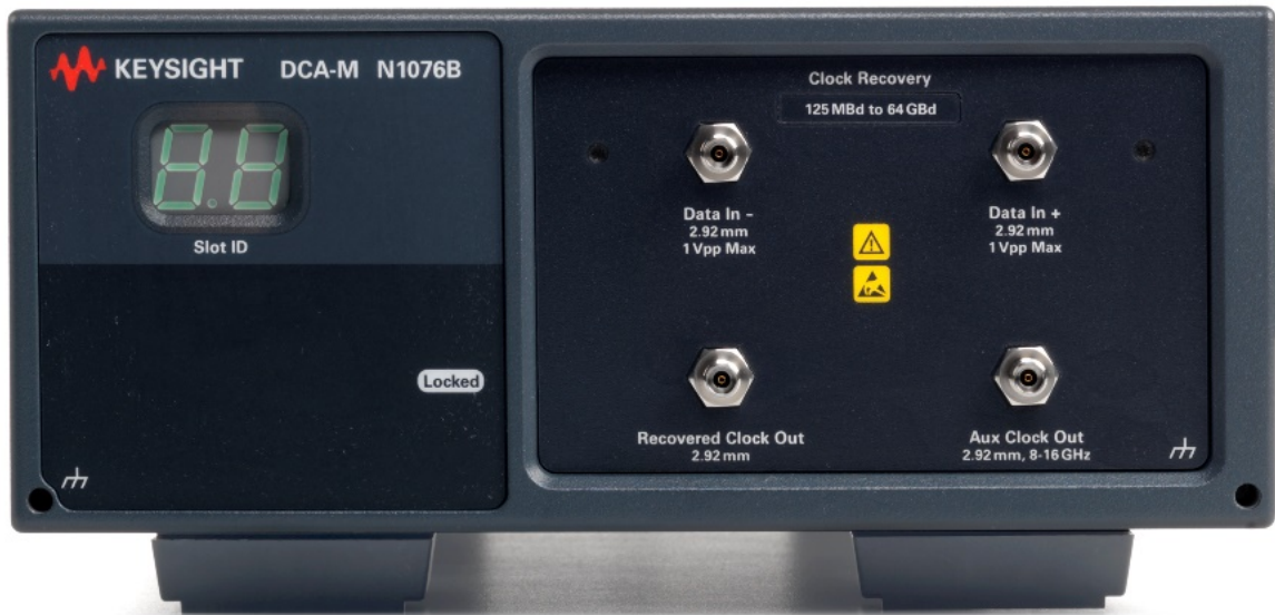
Figure 24: N1076B Electrical clock recovery with option 264
