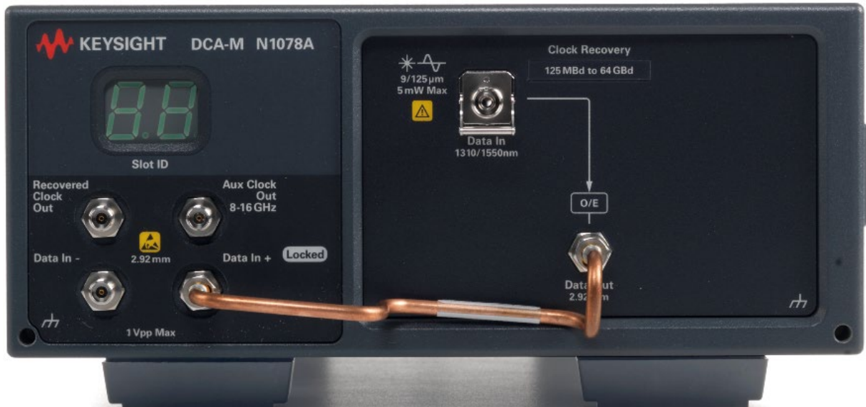
Figure 28: N1078A Single-mode optical/electrical clock recovery with options 264 and S50
