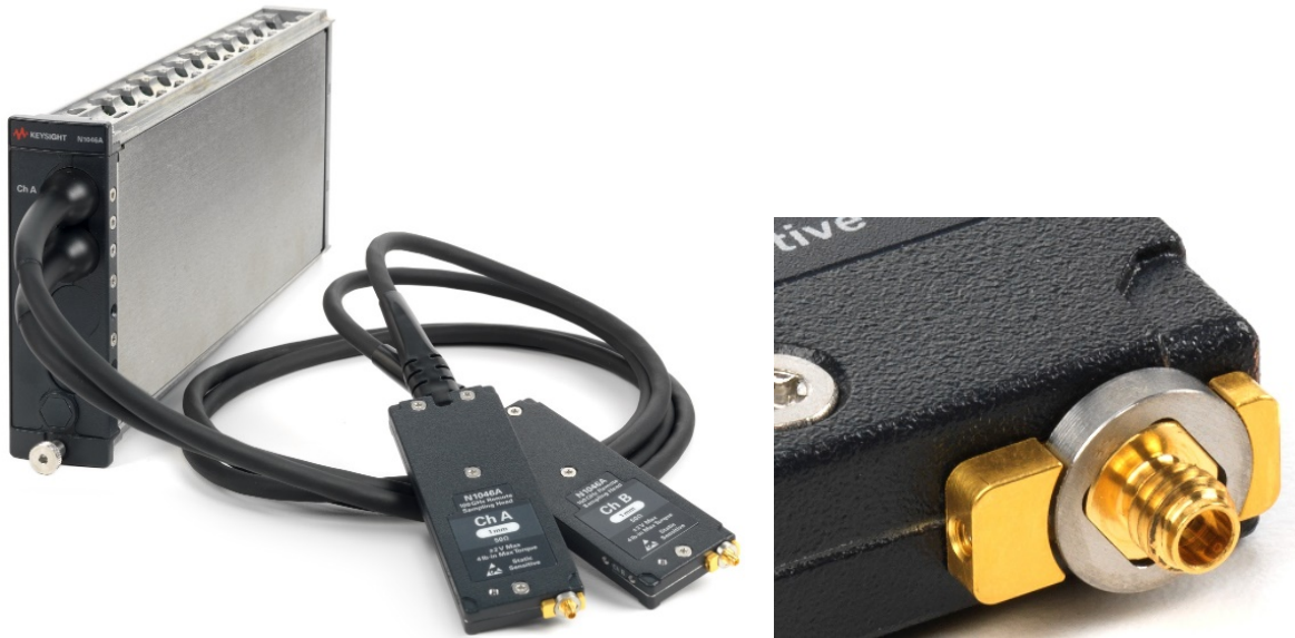
Figure 18: N1046A 100 GHz remote head module with option 12F, 1.0 mm input connector detail
