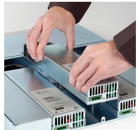
Figure 14d. User re-configurable modular system
