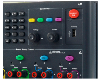
Figure 11. The N6705's front panel USB port.
