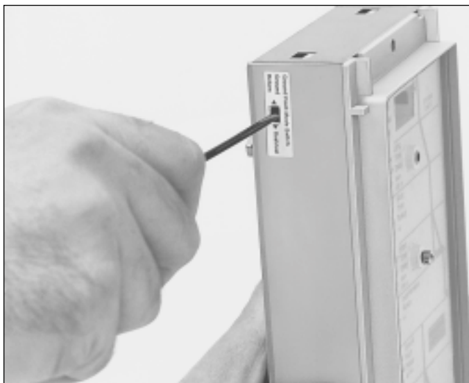
3. Set ground fault selection switch.
