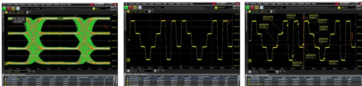
Figure 8. PAM-4 eye, level and rise/fall time measurements.
