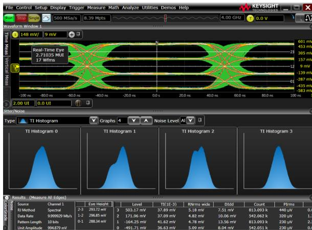
Figure 6. PAM-4 Noise Measurements
