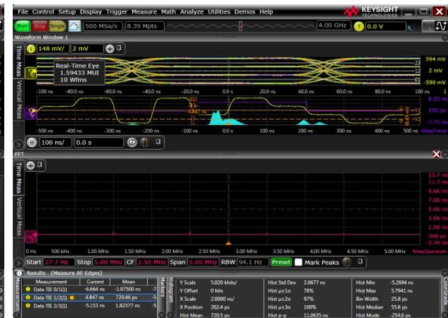
Figure 7. PAM-4 Jitter (Data TIE) Measurements
