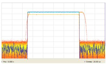
DPX Zero-span produces real-time analysis in amplitude, frequency, or phase vs. time. Up to 50,000 waveforms per second are processed. DPX Zero-span ensures that all time-domain anomalies are immediately found, reducing time-to-fault. Here, three distinct pulse shapes are captured in zero-span amplitude vs. time. Two of the three waveforms occur only once in 10,000 pulses, but all are displayed with DPX.
