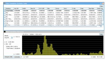
$\label{eq:cumulative statistics provides timestamps for Min, Max values as well as Peak to Peak,$ Average and Standard deviation over multiple acquisitions, further extending the analysis. Histogram shows you outliers on the right and left
