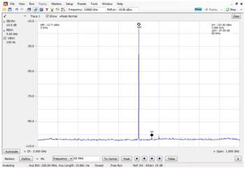
The wide-bandwidth, high dynamic range options (B85HD, B125HD, and B16xHD) offer unmatched real time spectrum analysis dynamic range. Two 16-bit, 200 MS/sec digitizers are interleaved, resulting in 400 MS/sec acquisitions with a typical spurious free dynamic range of -80 dBc, up to 10 dB better than other commercially available instruments. Here, a signal at 3 GHz is measured at -13.71 dBm, with the largest spurious signal from the digitizer -87.89 dB below the carrier.
