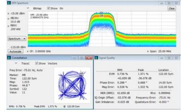
Time-correlated views in multiple domains provide a new level of insight into design problems not possible with conventional analyzers. Here, modulation quality and the constellation measurements are combined with the continuous monitoring of the DPX  $^{\mbox{\tiny 6}}$ spectrum display.
