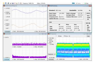
Analysis options for 802.11 standards are available. Here, an 802.11ac 160 MHz bandwidth signal is analyzed, with displays of EVM vs. subcarrier number and symbol number, channel response vs subcarrier with a summary of WLAN measurements, and the DPX spectrum of the analyzed signal. An EVM of -44.26 dB and other signal measurements are seen in the summary panel.
