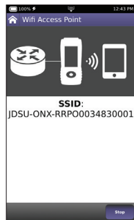
OneExpert DSL providing WiFi access point
