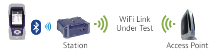
OneExpert DSL controls the Wifi Advisor for Single Ended Operation with Best Channel
