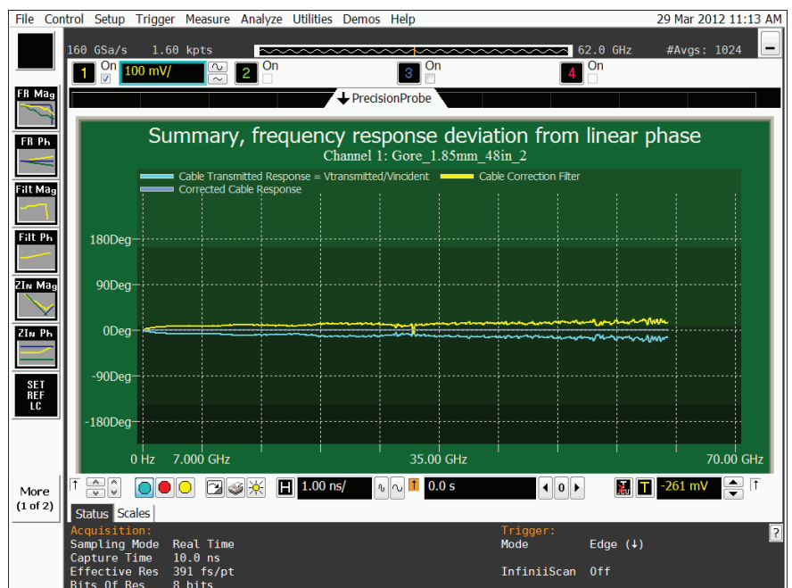
Figure 8. PrecisionProbe corrects phase non-linearities, notice the new flat phase.
