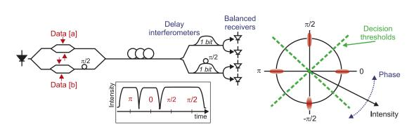
Figure 3: DQPSK - differential quadrature phase shift keying/differential detection
