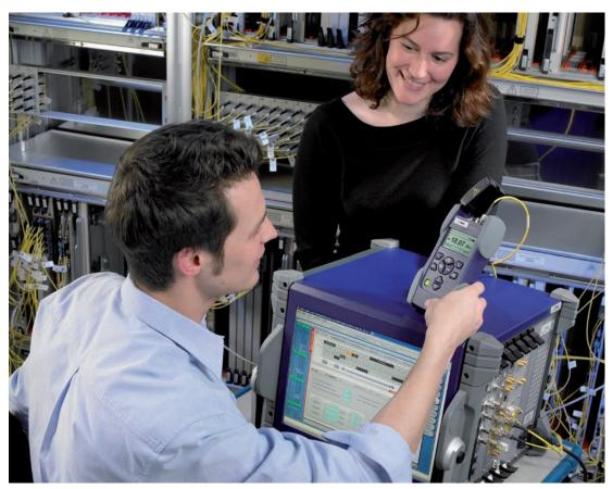
Figure 1: Using the ONT-506 to test modern DWDM systems
