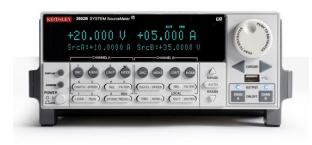
The Keithley 2636B is a 2600B series dual channel system SourceMeter® (SMU) instrument (0.1fA, 10A pulse). It is a leading current/voltage source and measure solution. This dual channel model combines the capabilities of a precision power supply, true current source, 6 1/2 digit DMM, arbitrary waveform generator, pulse generator and electronic load all into one tightly integrated instrument.
