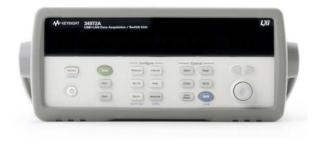
The Keysight 34970A data acquisition/data logger switch unit consists of a three-slot mainframe with a built-in 6 1/2 digit digital multimeter. Each channel can be configured independently to measure one of 11 different functions without the added cost or hassle of signal-conditioning accessories.
