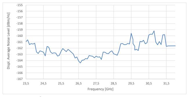
Measured at R&S®CMXHEAD30 remote radio head, RF1: displayed average noise level from 23.5 GHz to 31.8 GHz
