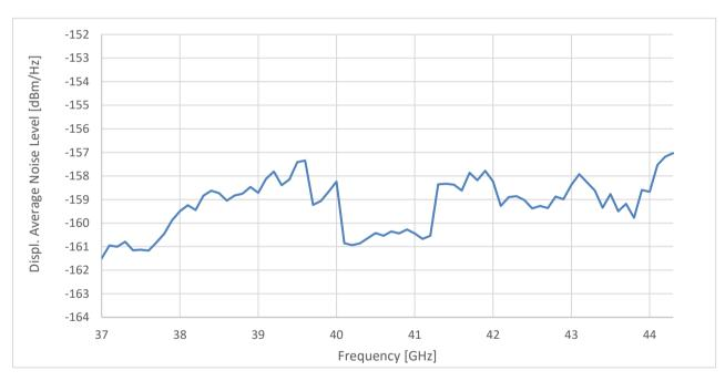
Measured at R&S®CMXHEAD30 remote radio head, RF1: displayed average noise level from 37 GHz to 44.3 GHz
