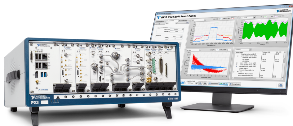
Figure 15. Integrated PXI Bench for FEM Test With DPD and Envelope Tracking.
