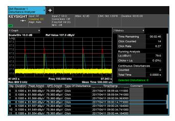
Figure 8. Simplify and automate data collection, analysis, and report generation for click measurements
