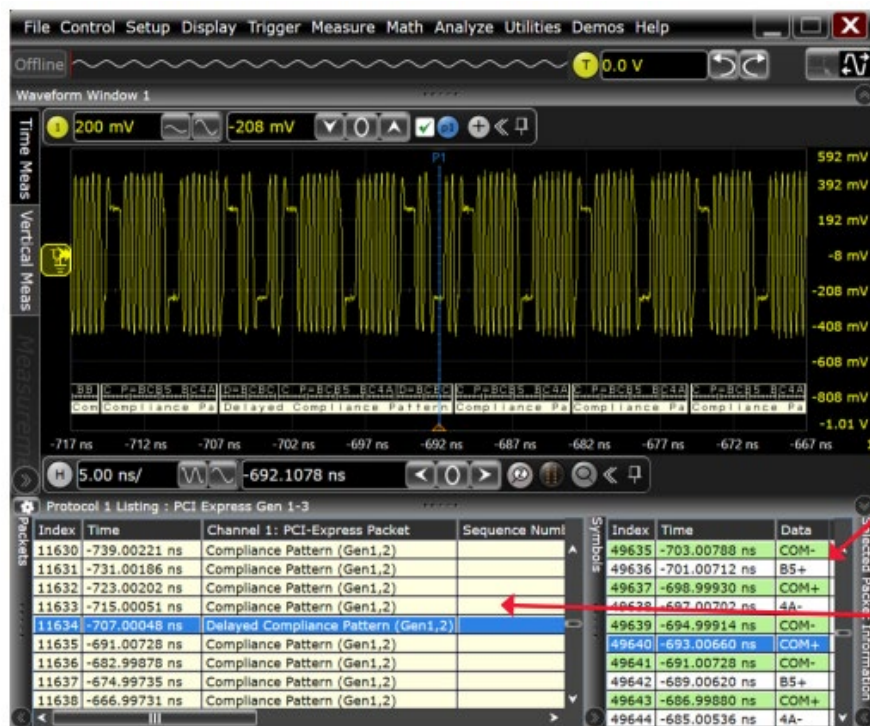
Figure 18. The N5463A provides 8b/10b and 128b/130b decode below
