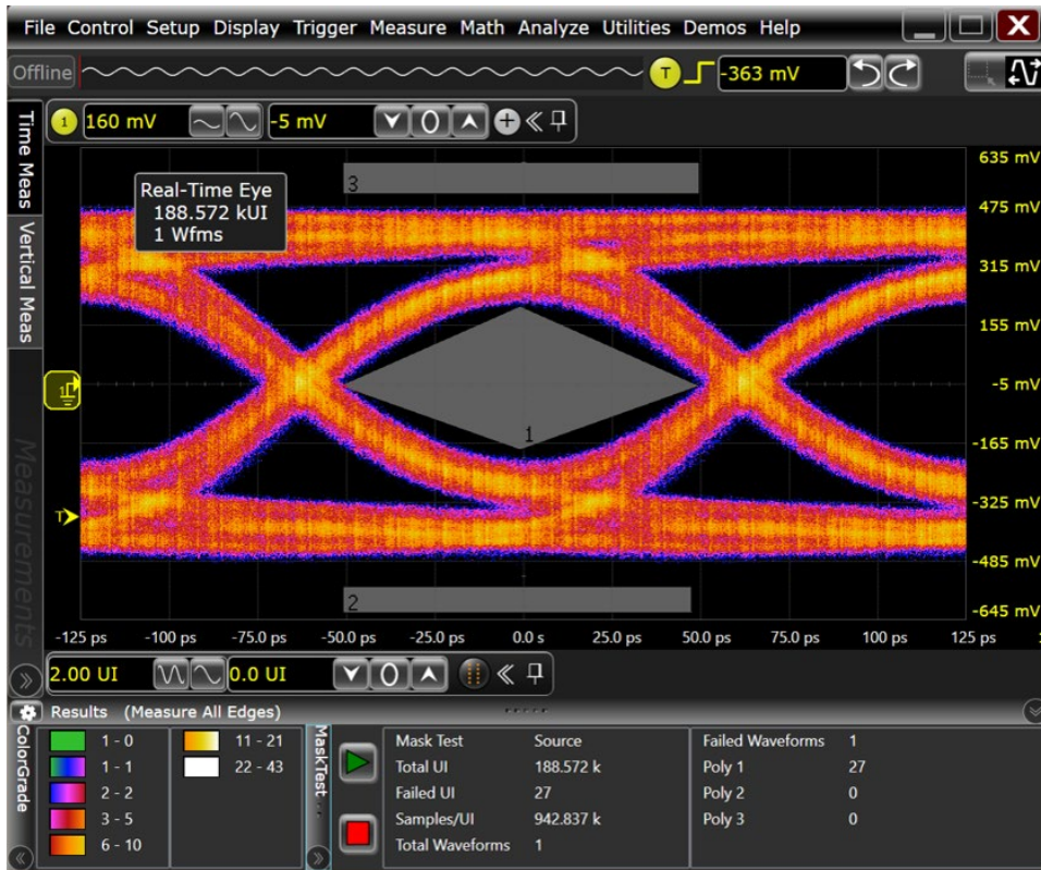
Figure 19. The Serial Data Analysis and optional D9020ASIA Equalization applications allow for the equalization of impaired 8 and 16 Gb/s signals so a clock can be recovered and mask testing can be performed on your waveforms
