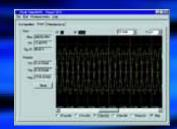
While the flowmeter can be fully set up via its integral keypad, the UltraScan program provides a simple and rapid means by which multiple flowmeters can be configured. In addition, the waveform analysis allows the user to easily determine the optimum location for transducer installation
