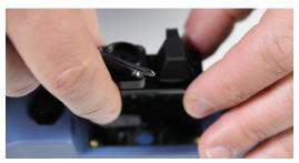
The power meter and VFL piece are offered as an easy-to-install option on the MAX-FIP display that's as simple as removing four screws.
