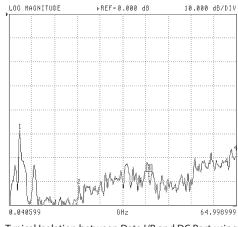
Typical Isolation between Data I/P and DC Port using Anritsu 37397C VNA
