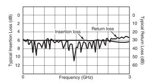
Insertion loss (typical) /return loss (typical)
