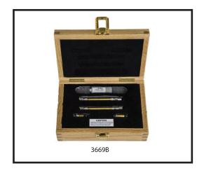
The Anritsu Verification Kits contain precision components with characteristics that are traceable to NIST. Used primarily by the metrology laboratory, these components provide the most dependable means of determining the system accuracy of your VNA. A disk containing factory measured test data for all components is supplied for comparison with customer-measured data.
