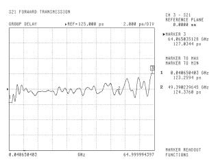
Typical Group Delay Performance measured on V255 using Anritsu 37397C VNA
