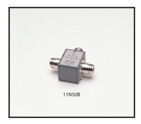
These RF power dividers are symmetrical, three-resistor tee designs that can be used in applications where signals from DC to 3000 MHz must be accurately divided. They are available in 50  $\Omega$ and provide excellent amplitude and phase tracking.
