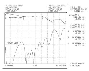
Insertion Loss and Return Loss measured on V261 over the range of 40 MHz to 65 GHz.
