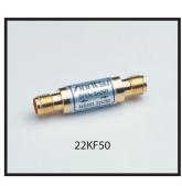
The 22 Series Open/Shorts are used on the test port of an SWR Autotester or SWR bridge to establish a full reflection reference for accurate SWR measurements. When used with scalar network analyzers, the open and short reflections over a swept frequency range can be automatically averaged to enhance measurement accuracy. All models consist of an open on one end and a short on the other.
