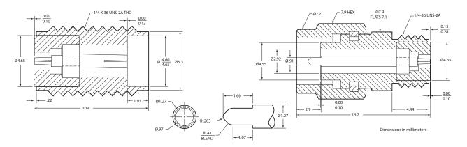
K Connector® interface dimensions in metric measurements
