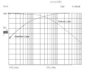
Typical Low Frequency Insertion Loss and Return Loss measured on K251 over the range of 1kHz to 1 MHz.
