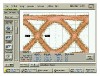
V265 Output Response to 2.0V NRZ Input Signal using Anritsu 43G ME7750A BERT
