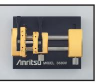
past, designers were forced to add extra line lengths, create one-of-a-kind custom fixtures, or worse, not test offset designs. With the flexibility of the 3680, you can test offset or in-line designs with one setup. Formerly-untestable designs can now be tested with ease.
