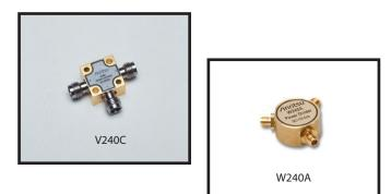
These microwave power dividers are symmetrical, three-resistor tee designs that can be used in applications where signals from DC to 65 GHz must be accurately divided or combined. K Connector<sup>®</sup> is compatible with 3.5 mm and SMA; V Connector<sup>®</sup> is compatible with 2.4 mm. All models have exceptional amplitude and phase tracking characteristics.
