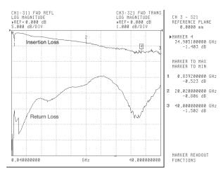
Typical Frequency Insertion Loss and Return Loss measured on K251 over the range of 40 MHz to 40 GHz.
