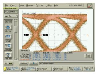
Input Test Signal to V265 2.0 V NRZ Input Signal using Anritsu 43G ME7750A BERT
