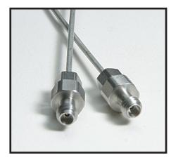
The W1 Connector<sup>\*</sup> family is a complete coaxial connector system with mode-free performance to 110 GHz. Based on the 1.00 mm coaxial connector front side interface as specified by IEEE Std 287, the W1 Connector is well suited for high frequency applications ranging from components to systems and instrumentation.
