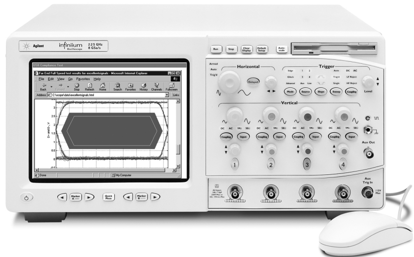
Figure 8. The USB option eliminates the need to transfer data to a PC for post-processing.
