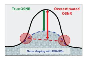
Therefore, Viavi developed a proprietary method for measuring OSNR within the signal bandwidth that shows the true in-band OSNR. Unlike other solutions, the Viavi instrument measures and displays the noise distribution for the entire width of each DWDM channel to measure the signal's true OSNR.
