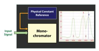
Excessive channel wavelength drift in DWDM systems can degrade performance and increase bit error rates because of high power attenuation in network elements such as multiplexers, demultiplexers, and ROADMs. Although it requires high wavelength accuracy, an OSA can detect this problem.
