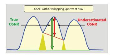
Introducing ROADMs further complicates measuring OSNR with the conventional methods described in
