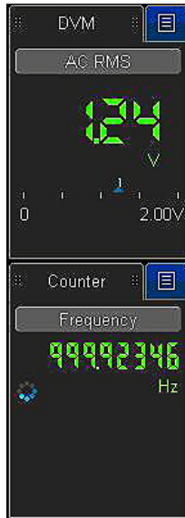
Figure 25. DVM and counter takes advantage of separate signal paths to provide measurements without a trigger, while still using the scope probes.
