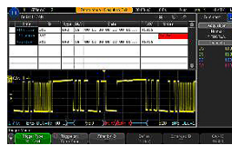
Figure 17. CAN-FD decode and trigger.
