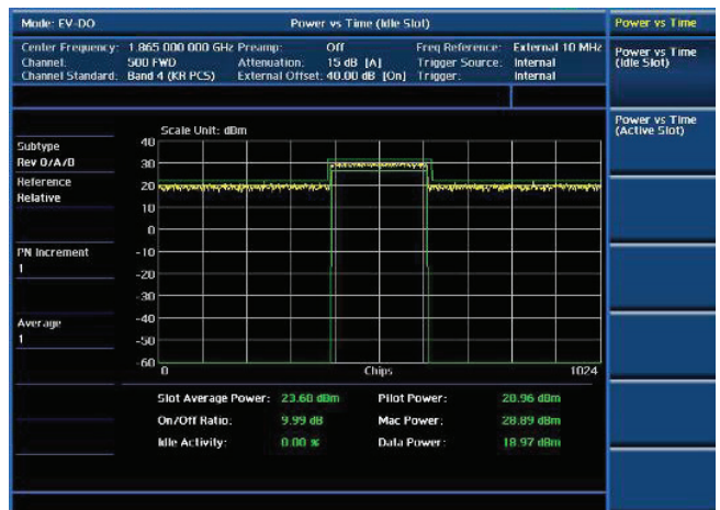
EV-DO power vs. time (idle slot)
