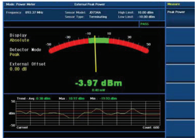
External power measurement
