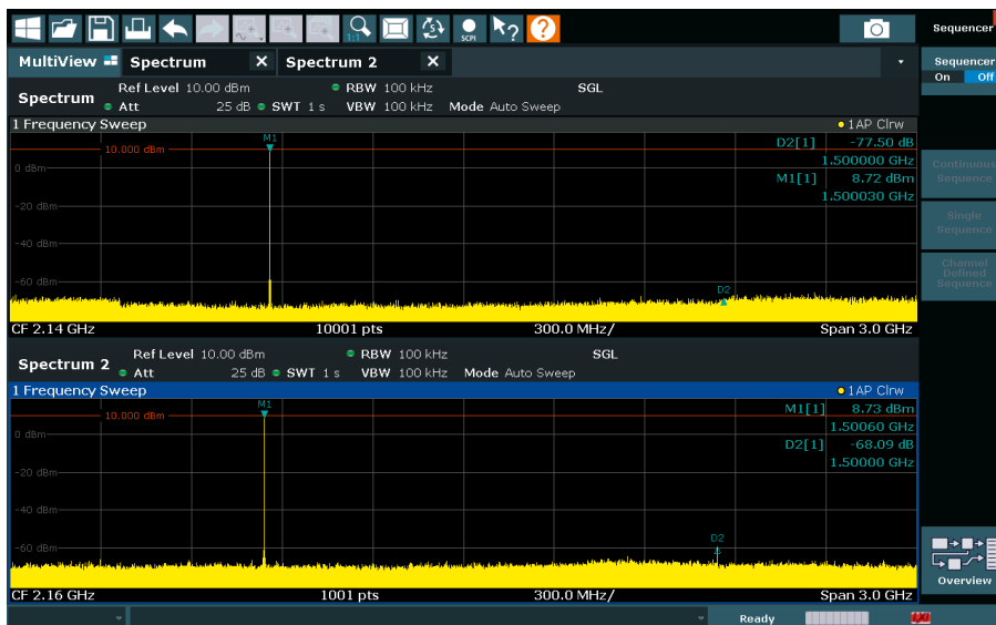
Harmonic measurement with highpass filter switched on (top) and off (bottom)
