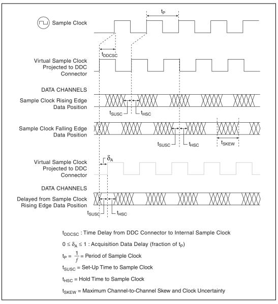
Figure 3. Acquisition Timing Diagram
