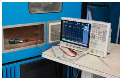
N7013A allows the use of differential probe inside an environmental chamber for extreme temperature testing
