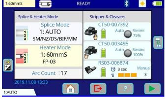
\*Basic operations can be performed from the touch screen after the power is turned on.
