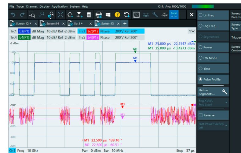
Pulse profile measurement with arbitrary pulse sequences. Pulse sequences can be measured on multiple receivers simultaneously. Since the receivers are phase coherent, they not only measure the amplitude of a pulse but also its phase with high stability. This allows the phase deviation of a DUT to be determined very simply and reliably.
