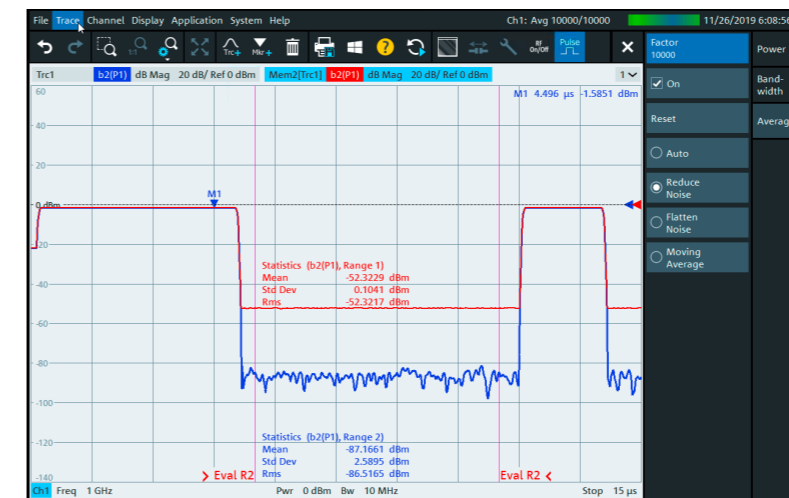
Pulse profile measurement: the wideband measurement mode enables single-shot pulse sweeps without averaging. Averaging (AVG) modes are also available to achieve either a very low trace noise or a very high dynamic range (i.e. a high pulse on/off ratio) based on vector averaging. Red trace: AVG mode "flatten noise". Blue trace: AVG mode "reduce noise".
