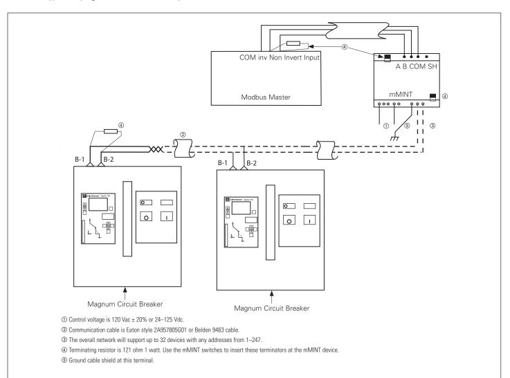
Figure 51. Modbus Translator Wiring
