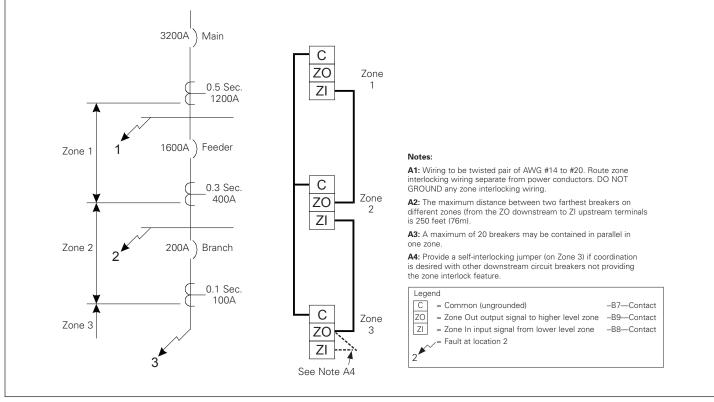
Figure 48. Typical Zone Interlocking
