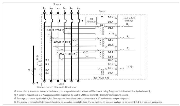
Figure 12. Source Ground Fault Sensing Scheme for 4000A Frame—Double-Wide
