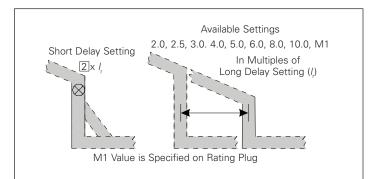
Figure 33. Short Delay Current Settings
