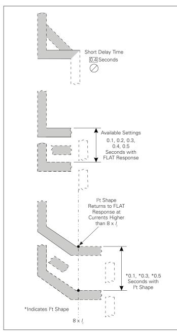
Figure 34. Short Delay Time Settings
