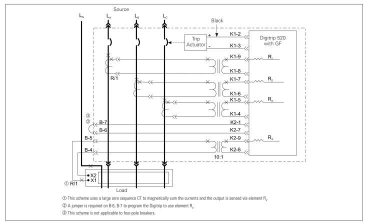
Figure 13. Zero Sequence Sensing Scheme for 3200A Frame
