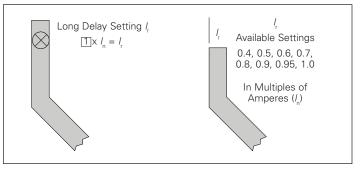
Figure 30. Long Delay Current Settings
