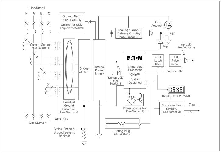
Figure 15. Block Diagram with Breaker Interface
