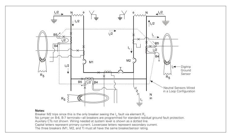
Figure 14. Multiple Source/Multiple Ground Scheme
