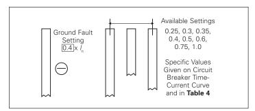
Figure 36. Ground Fault Current Settings
