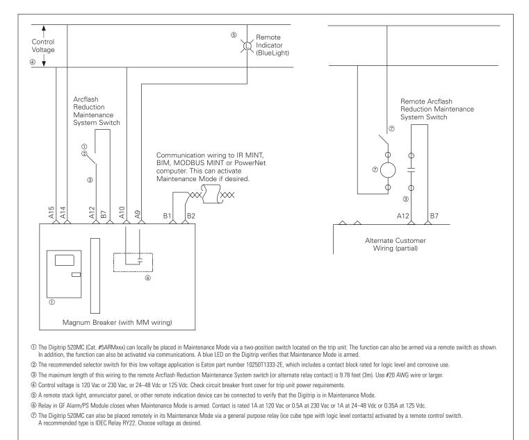
Figure 47. Maintenance Mode Wiring—Digitrip 520MC
