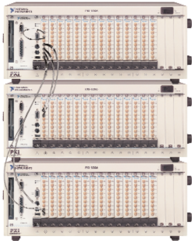
Figure 6. In this example, three PXI chassis containing 13 PXI-4472 eight-channel 102.4 kS/s simultaneous-sampling dynamic signal acquisition modules are synchronized. The result is a 312-channel synchronized acquisition system.
