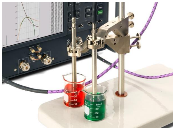
Figure 7. Two port configuration with PNA and performance probe kit
