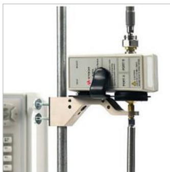
Figure 2. Ecal module connected in line for electronic calibration refresh.
