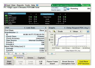
Figure 12. IEEE 1588v2 PTP configuration test results
