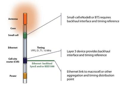
Figure 1. A typical small-cell site configuration
