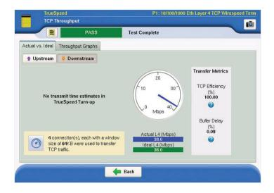
Figure 11. RFC 6349 TrueSpeed TCP throughput results
