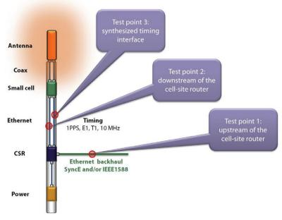
Figure 2. Small-cell test points
