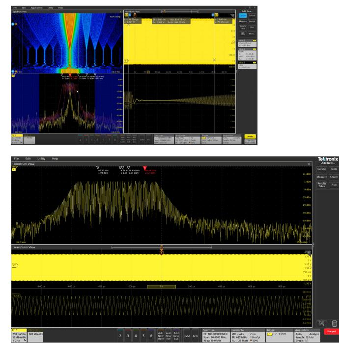
The lower trace is the frequency vs. time trace derived from the input signal. Notice that the Spectrum Time is positioned during a transition from the lowest frequency to the middle frequency, so the energy is spread across a number of frequencies. With the frequency vs. time trace, you can easily see the different frequency hops, simplifying characterization of how the device switches between frequencies.
