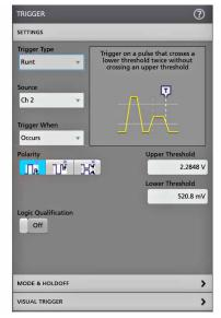
Configuration menus are accessed by simply double-tapping on the item of interest on the display. In this case, the Trigger badge was double-tapped to open the Trigger configuration menu.
