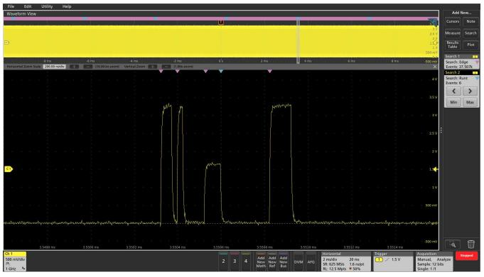
Earlier, FastAcq revealed the presence of a runt pulse in a digital data stream prompting further investigation.
