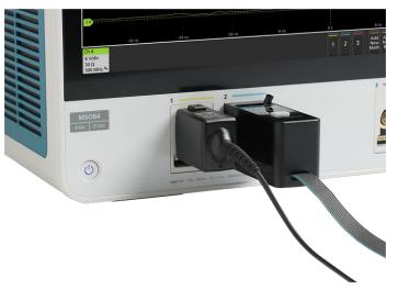
FlexChannel technology enables the ultimate in flexibility. Each input can be configured as a single analog or eight digital channels based on the type of probe you attach.
