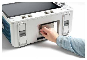
When the SSD is present, the instrument boots in an open Windows 10 configuration, so you can minimize the oscilloscope application and access a Windows desktop where you can install and run additional applications on the oscilloscope or you can connect additional monitors and extend your desktop.
