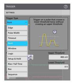
The wide variety of trigger types and context-sensitive help in the trigger menu make it easier than ever to isolate the event of interest.
