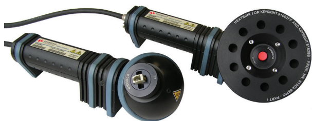
81628B InGaAs head with integrating sphere
