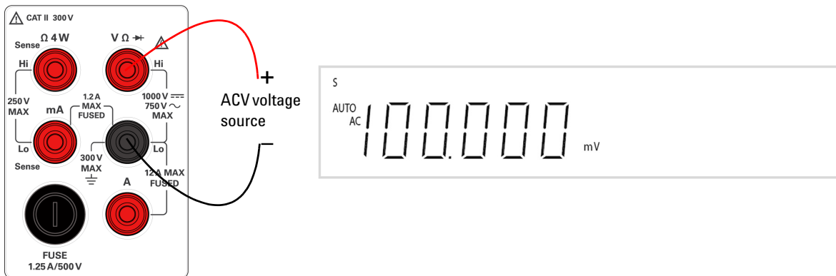
Figure 1-10 ACV terminal connection and display
