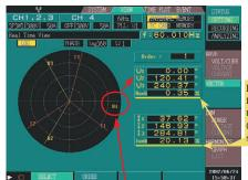
Displays the unbalance factor when measuring three-phase power lines. (For 3P3W3M and 3P4W settings)
