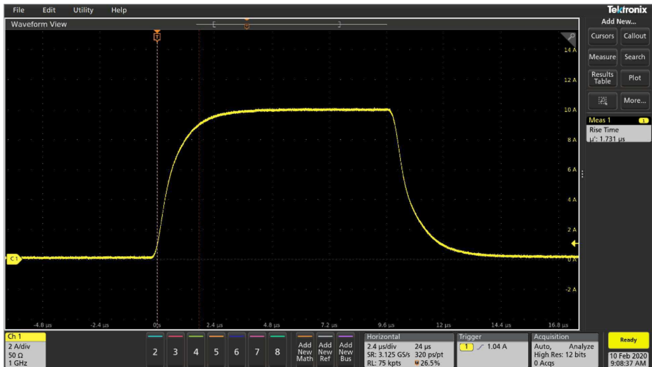
Pulse output performance of the 2610B-PULSE SMU.
