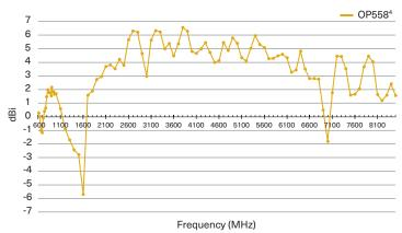
$<sup>^4</sup>$  Measured connected directly to IBflex $^8$  scanning receiver, which provides a ground plane of 4.4" x 1.55" (112 mm  $\,$  x 39 mm).
