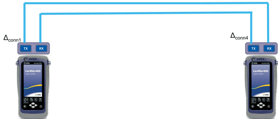
Figure 2. Loss measurement = fiber system under test + \Delta_{\text{conn2}} + \Delta_{\text{conn3}} . Limit = \Delta_{\text{conn2}} + \Delta_{\text{conn3}} @ 0.75 dB each + connection/splice/length loss for the fiber system under test
