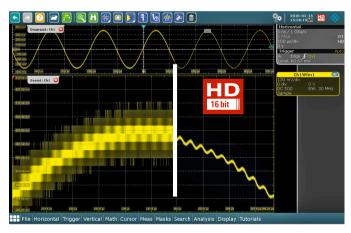
The 16-bit HD mode makes signals details visible that are otherwise hidden in noise
