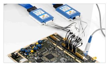
Every R&S®RTP can be upgraded on site with 16 digital channels
