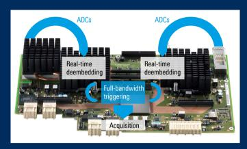
R&S®RTP real-time deembedding and trigger board
