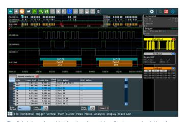
The digital channels are ideal for triggering and decoding low-speed serial interfaces such as SPI
