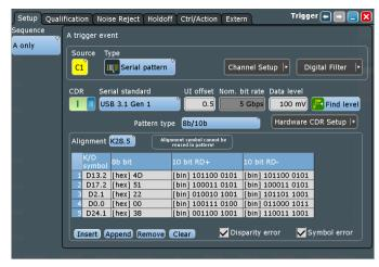
Setup dialog for the high speed serial pattern trigger
