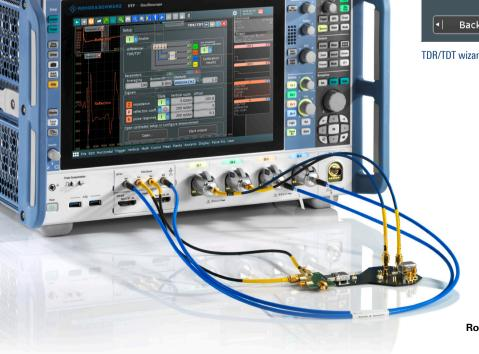
Differential test setup with the R&S®RTP-B7 pulse source and the R&S®RTP-K130 TDR/TDT analysis option
