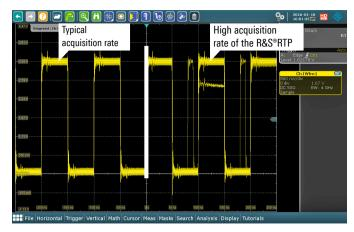
The high acquisition rate detects sporadic signal faults fast
