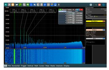
Display of EMI measurement results on a logarithmic y-axis
