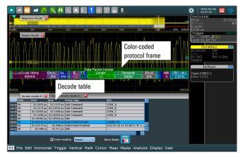
Clear display of decoded data in the waveform and in the decode table
