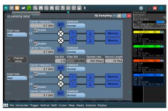
Setup dialog for the R&S®RTP-K11 I/Q interface
