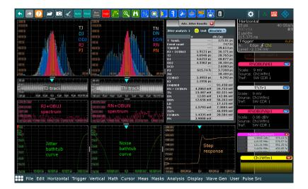
Displays the step response, individual jitter and noise components in histograms, spectrum, synthetic eye diagram and BER bathtub curve of an 8 Gbps PCIe Gen3 signal.
