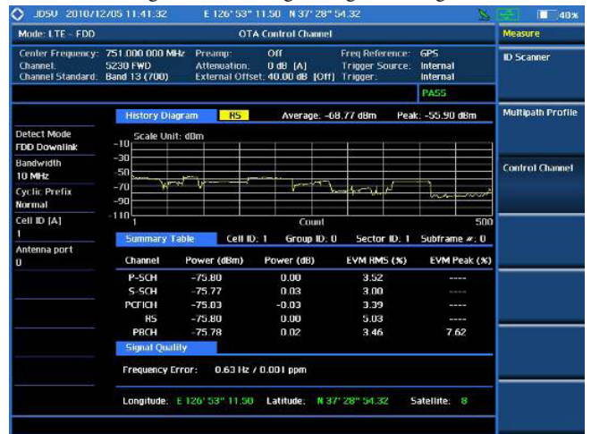
LTE OTA control channel
