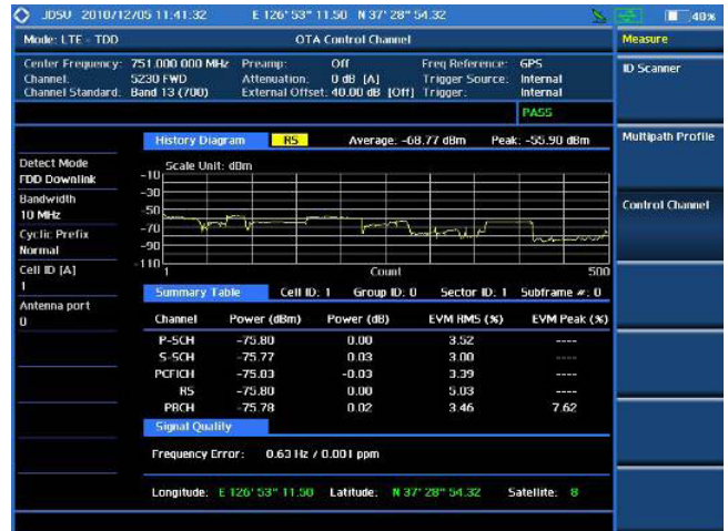
LTE OTA control channel
